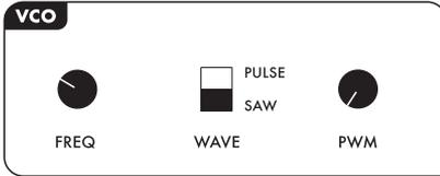
The keyboard determines the note played based on the setting of the Freq control - these two control inputs are summed together.
