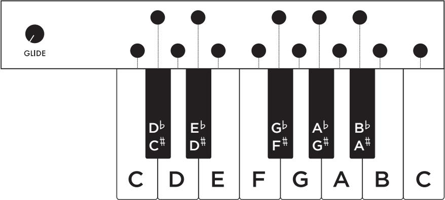
This diagram shows how the “button” keyboard of the Werkstatt (above) relates to a standard piano keyboard. Although the note names shown are correct for this layout, the actual note being produced will also depend on many factors, including the VCO FREQ knob, etc...
